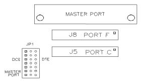
Figure 3. Master Port DCE/DTE Jumpers
